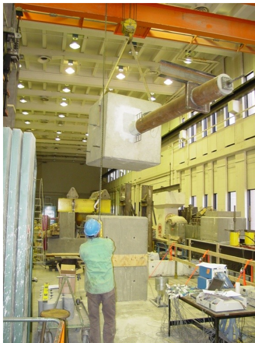
Figure 4-19- Placing specimen #1 on top of support blocks
