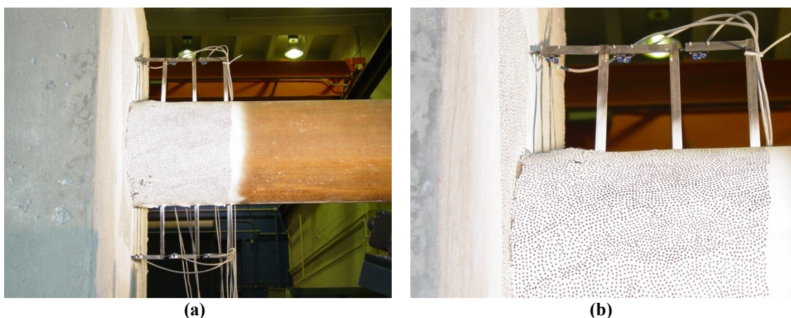
Figure 4-25- (a) Excessive deformation near the first gages at load stage 3-16 ( \pm 3.00 in) (b) large deformation around the rod holding PT1
