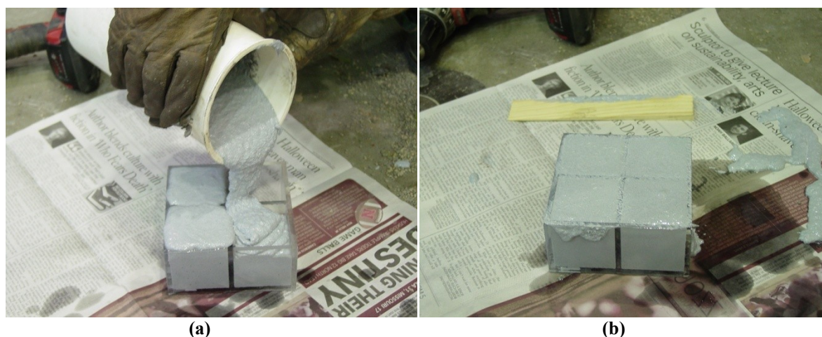
Figure 4-68- (a) Pouring the mix (b) leveled top surface
